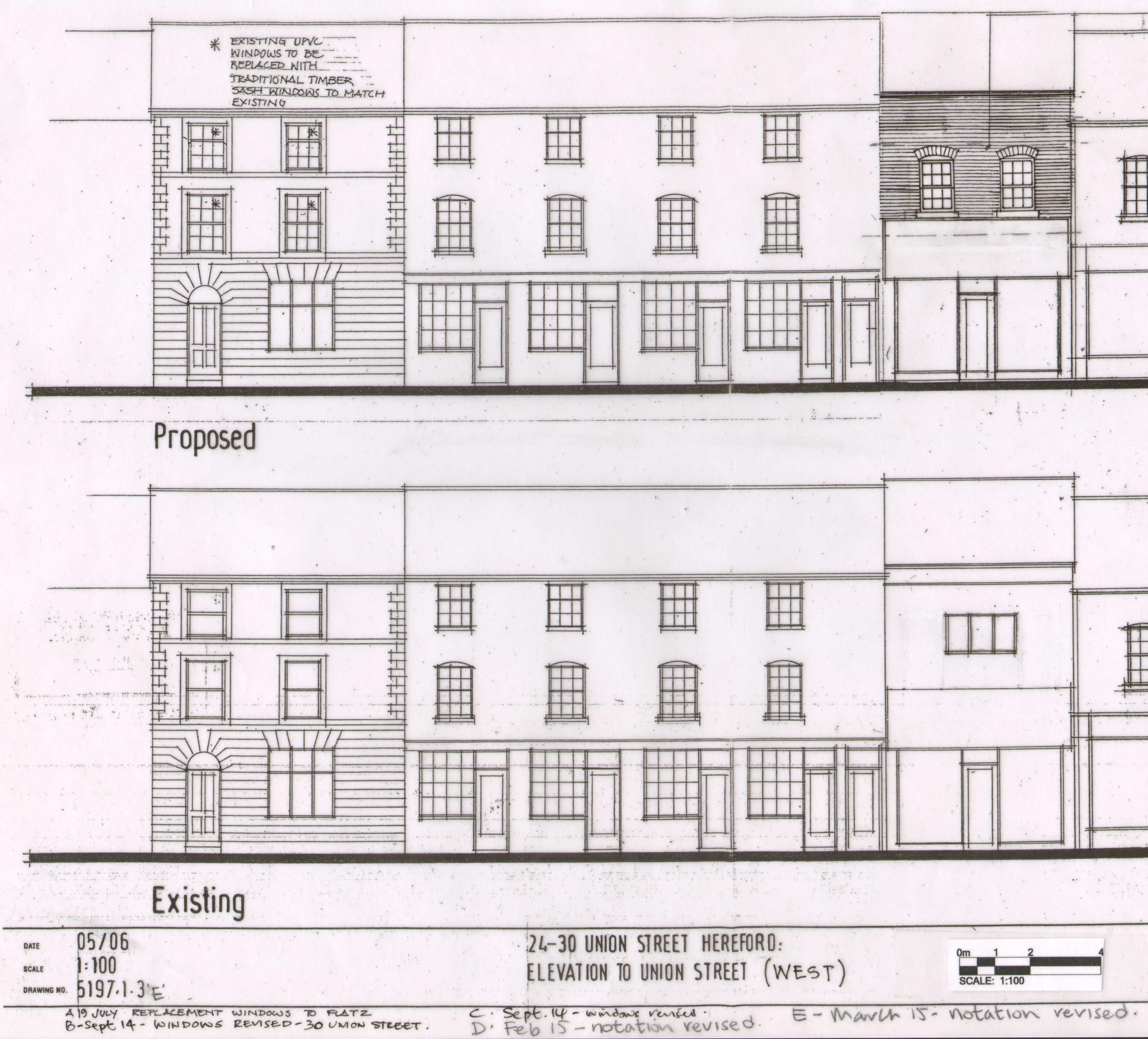
& part signage fascia. Rebuild brickwork as necessary behind & incorporate two timber sliding sash windows at first floor level.
